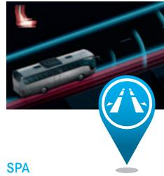
The lane departure warning system (SPA) alerts the driver prior to unintentional departure from a lane through clearly noticeable vibration of the surface of the driver's seat on the side corresponding to the lane marking that has been crossed.
