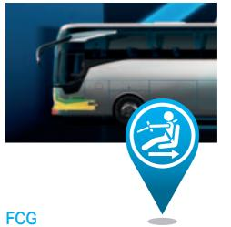
The front collision guard (FCG) consists of crash elements which, in the event of a collision, selectively dissipate energy and can prevent a car from going under the vehicle. In addition, the driver's station, including steering, pedals and seat, is displaced to the rear as a complete unit in the event of a serious head-on collision, thereby increasing the survival space by vital centimetres.
