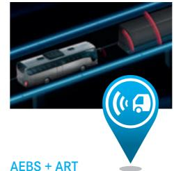
The advanced emergency braking system (AEBS) initiates partial and full braking as part of an ascending scale of warnings to avoid a rear-end collision. In order to completely avoid an accident, adaptive cruise control (ART) detects any vehicle driving slower in front or a stationary obstacle in good time with a distance sensor and automatically brakes the coach by the time a predefined distance is reached (which it consistently maintains).
