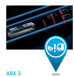
The Active Brake Assist 3 system (ABA 3) warns the driver if the defined distance from a vehicle driving in front or a stationary obstacle is too short, initiating partial or full braking if the driver fails to react.
