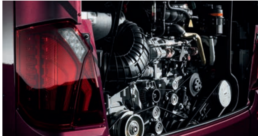
Tested and proven on more than 60 million kilometres: The Mercedes-Benz BlueEfficiency OM 471 power engine achieves a power output of 375 kW (510 hp). The compact unit is designed for low operating costs and low exhaust emissions. At the same time, it achieves impressive driving dynamics with its high torque. Extremely long oil change intervals of up to 120,000 kilometres ensure favourable maintenance costs.
